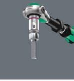
The clamping of the screw is achieved by a flexible locking ball. The holding function is especially helpful in confined, hard-to-reach spaces, where there is no room for a second hand to secure the screw. Manual and machine sockets
