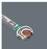
The Joker's clever double-hex geometry delivers a very positive connection with nuts or bolts – it's a perfect fit. And the exchangeable, hardened metal gripping plate in the Joker's mouth literally bites itself into the bolt, with its extremely hard tips. Both features combine to prevent slipping, even at higher torque.
