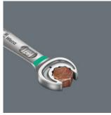
The Joker's clever double-hex geometry delivers a very positive connection with nuts or bolts - it's perfect fit. And the а exchangeable, hardened metal gripping plate in the Joker's mouth literally bites itself into the bolt, with its extremely hard tips. Both features combine to prevent slipping, even at higher torque.
