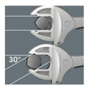
Thanks to the corner-width rectangular prisms, a return angle of only 30° can be realized.
