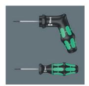
Wera torque-indicators have been factory pre-set to values recommended by leading carbide manufacturers. tool These tightening values relate specifically to the size of the TORX®, TORX PLUS® or hexagon socket screw. Torque indicators ensure safe and screw easy loosening of connections. Precision: ± 10 %
