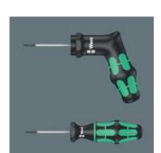
Wera torque-indicators have been factory pre-set to values recommended by leading carbide manufacturers. tool These tightening values relate specifically to the size of the TORX®, TORX PLUS® or hexagon socket screw. Torque indicators ensure safe and easy loosening of screw connections. Precision :  $\pm$  10 %
