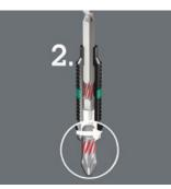
Higher peak loads are minimised through the torsion effect of the bit shaft (Phase 2). This effect is achieved with a specific heat treatment after the hardening process of the bits. This reduces the hardness of the shaft in comparison to the drive tip.
