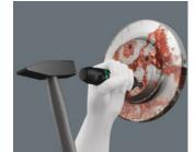
Seized screws can be loosened or tightened without power tools.
