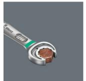
The Joker's clever double-hex geometry delivers a very positive connection with nuts or bolts - it's fit. And perfect exchangeable, hardened metal gripping plate in the Joker's mouth literally bites itself into the bolt, with its extremely hard tips. Both features combine to prevent slipping, even at higher torque.
