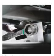
With the Joker, you can now loosen and tighten nuts and bolts, in situations where conventional tools fail. Particularly in confined spaces, where conventional open-jawed wrenches cannot be used. The combination of limit stop and small return angle enables eff ective work, even on screw pipe connections.
