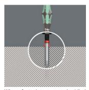
When fastening screws in blind holes the screw gripper is pushed back, making it possible to reach even deep-seated screws.
