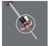
Pull the screw gripper towards the screwdriver handle until the two arms of the gripper sit against the head of the screw and are spread slightly apart. The Wera screw gripper releases the screw automatically after it has been fastened.
