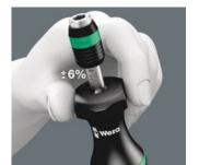
Measurement accuracy is  $\pm$  6 % in accordance with the standard DIN EN ISO 6789. Distinctly audible and noticeable excess-load signal when the pre-set torque is reached.
