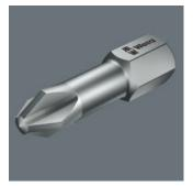
TZ-Bits are tough viscous bits with a torsion zone. Torsion bits absorb the damaging peak torque loads in the torsion zone. This prevents premature wear and enhances the service life of the bits.
