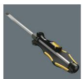
A hexagon blade made out of highquality bit material extends right through the handle - thereby ensuring full transfer of force, even when struck with a hammer. The ductile tempered material prevents the blade from splintering or breaking. Kraftform Plus – Series 900
