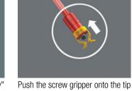
of the screwdriver until the end of the blade protrudes from the rubber blade holder.
