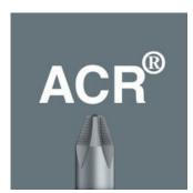
ACR® stands for "anti-cam-out ribs". ACR® bits have ribs at the drive tip that protect against slipping out of the screw head. It is recommended that ACR® bits are matched with ribbed ACR® screws for maximum effect. ACR® is a registered trademark of Phillips Screw Company.
