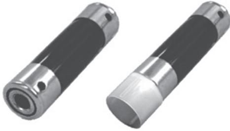
Rugged, precision machined end pieces are held in place by heavy steel collars. Set screws at each end insure that there is no slippage on the shaft flats. Quiet, noise and vibration absorbing, these premium couplings out-perform conventional couplings where misalignment exists or where punishing service is the norm. Available for 1/2" x 7/16" and 1/2" x 5/16" shaft sizes, or 7/16" shaft x spline socket.
