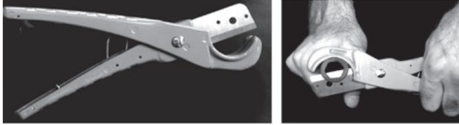
Cuts coupling shafts quickly and cleanly. No twisting or turning necessary. Cuts 1/8" to 1-1/4" O.D. rubber, polyethylene, neoprene, vinyl, PVC, etc. Reversible blade gives twice the blade life. Curved handles are easy on the hands.
