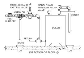
3. Under certain backflow conditions, the Model 760 will spill water from the vent port.
