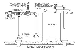
3. Under certain backflow conditions, the Model 760 will spill water from the vent port.
