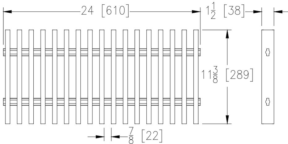
**GG GRATE ENGINEERING SPECIFICATION:** The Zurn P12-GG Vinylester Fiberglass Slotted Grate, is 11-3/8" [289mm] wide X 24" [610mm] long, weighing 2.8 lbs per linear foot [4 kg/m]. The grate has an open area of 82.5 in<sup>2</sup> per linear foot [1746 cm<sup>2</sup>/m], DIN Rating of A, ANSI Rating of Light-Duty and a slip resistant surface. Conforms to interplastic CORVE8300, or REICHHOLD DION 9100, or equivalent.
