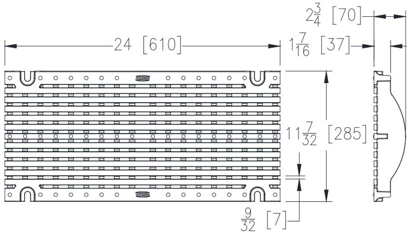
**HPDE GRATE ENGINEERING SPECIFICATION:** The Zurn P12-HPDE Ductile Iron Heel-Proof Longitudinal Grate, is 11-7/32" [285mm] wide X 24" [610mm] long, weighing 29.6 lbs per linear foot [44 kg/m]. The grate has an open area of 29.9 in<sup>2</sup> per linear foot [633 cm<sup>2</sup>/m], DIN Rating of E, ANSI Rating of Special-Duty, ADA compliant, H-20 Load Rated, and FAA Load Rated. Ductile Iron conforms to ASTM A536 Grade 80-55-06.
