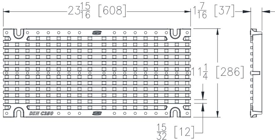
**ADA-USA GRATE ENGINEERING SPECIFICATION:** The Zurn P12-ADA-USA Ductile Iron Grate, is 11-1/4" [286mm] wide X 23-15/16" [608mm] long, weighing 15.6 lbs per linear foot [23kg/m]. The grate has an open area of 65.2 in<sup>2</sup> per linear foot [1380 cm<sup>2</sup>/m], DIN Rating of C, ANSI Rating of Heavy-Duty, ADA compliant, and H-20 Load Rated. Ductile Iron conforms to ASTM A536 Grade 80-55-06.
