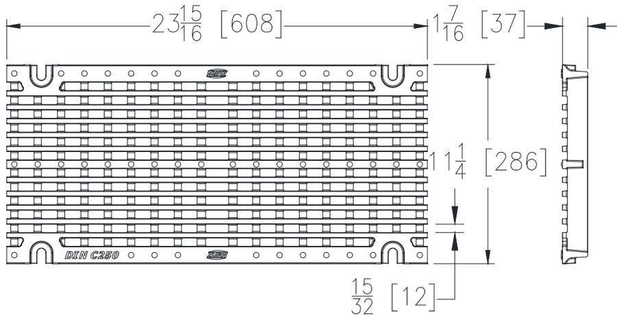
**GADA-USA GRATE ENGINEERING SPECIFICATION:** The Zurn P12-GADA-USA Galvanized Ductile Iron ADA Compliant Grate, is 11-1/4" [286mm] wide X 23-15/16" [608mm] long, weighing 15.6 lbs per linear foot [23 kg/m]. The grate has an open area of 65.2 in<sup>2</sup> per linear foot [1380 cm<sup>2</sup>/m], DIN Rating of C, ANSI Rating of Heavy-Duty, ADA compliant, and H-20 Load Rated. Ductile Iron conforms to ASTM A536 Grade 80-55-06. Galvanizing (hot dip) conforms to ASTM specification A123.
