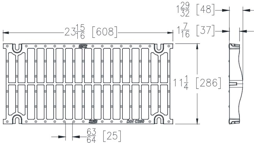
**BDC GRATE ENGINEERING SPECIFICATION:** The Zurn P12-BDC Black Acid Resistant Epoxy Coated Ductile Iron Slotted Grate, is 11-1/4" [286mm] wide X 23-15/16" [608mm] long, weighing 14.7 lbs per linear foot [22 kg/m]. The grate has an open area of 86.7 in<sup>2</sup> per linear foot [1835cm<sup>2</sup>/m], DIN Rating of C, ANSI Rating of Heavy-Duty, and H-20 Load Rated. Ductile Iron conforms to ASTM A536 Grade 80-55-06.
