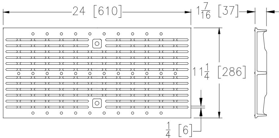
**HPD GRATE ENGINEERING SPECIFICATION:** The Zurn P12-HPD Ductile Iron Heel-Proof Longitudinal Grate, is 11-1/4" [286mm] wide X 24" [610mm] long, weighing 14 lbs per linear foot [21 kg/m]. The grate has an open area of 33.7 in<sup>2</sup> per linear foot [713 cm<sup>2</sup>/m], DIN Rating of B, ANSI Rating of Medium-Duty, and ADA compliant. Ductile Iron conforms to ASTM A536 Grade 80-55-06.
