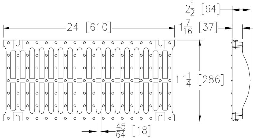
**DGF GRATE ENGINEERING SPECIFICATION:** The Zurn P12-DGF Ductile Iron Slotted Grate, is 11-1/4" [286mm] wide X 24" [610mm] long, weighing 26 lbs per linear foot [39 kg/m]. The grate has an open area of 54 in<sup>2</sup> per linear foot [1143 cm<sup>2</sup>/m], DIN Rating of F, ANSI Rating of Special-Duty, H-20 Load Rated, and FAA Load Rated. Ductile Iron conforms to ASTM A536 Grade 80-55-06.
