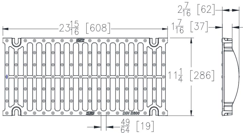
**GDE GRATE ENGINEERING SPECIFICATION:** The Zurn P12-GDE Galvanized Ductile Iron Slotted Grate, is 11-1/4" [286mm] wide X 23-15/16" [608mm] long, weighing 19.8 lbs per linear foot [29 kg/m]. The grate has an open area of 60.3 in<sup>2</sup> per linear foot [1276 cm<sup>2</sup>/m], DIN Rating of E, ANSI Rating of Special-Duty, H-20 Load Rated, and FAA Load Rated. Ductile Iron conforms to ASTM A536 Grade 80-55-06. Galvanizing (hot dip) conforms to ASTM specification A123.
