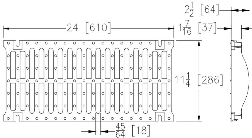
**GDF GRATE ENGINEERING SPECIFICATION:** The Zurn P12-GDF Galvanized Ductile Iron Slotted Grate, is 11-1/4" [286mm] wide X 24" [610mm] long, weighing 26 lbs per linear foot [39 kg/m]. The grate has an open area of 54 in<sup>2</sup> per linear foot [1143 cm<sup>2</sup>/m], DIN Rating of F, ANSI Rating of Special-Duty, H-20 Load Rated, and FAA Load Rated. Ductile Iron conforms to ASTM A536 Grade 80-55-06. Galvanizing (hot dip) conforms to ASTM specification A123.
