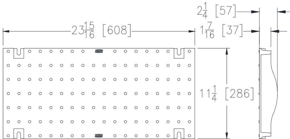
**DC COVER ENGINEERING SPECIFICATION:** The Zurn P12-DC Ductile Iron Solid Cover, is 11-1/4" [286mm] wide X 23-15/16" [608mm] long, weighing 27.9 lbs per linear foot [42 kg/m]. The solid ductile iron cover has a DIN Rating of E, ANSI Rating of Special-Duty, ADA Compliant, H-20 Load Rated and FAA Load Rated. Ductile Iron conforms to ASTM A536 Grade 80-55-06.
