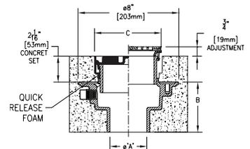
\*Cast Iron Adapter substituted for standard ABS adapter
