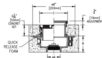
\*Cast Iron Adapter substituted for standard ABS adapter
