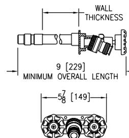
Standard inlet connection combination 1/2" [13mm] female solder x 1/2" [13mm] male IP.
