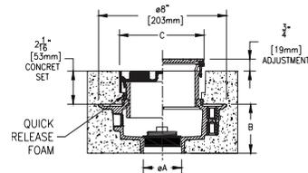
\*Cast Iron Adapter substituted for standard ABS adapter
