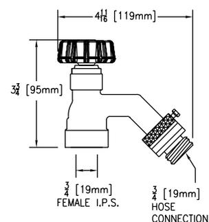
Standard inlet connection 3/4" [19mm] female pipe thread.
