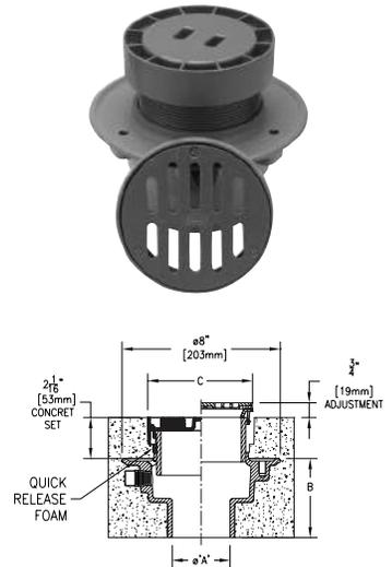
\*Cast Iron Adapter substituted for standard ABS adapter
