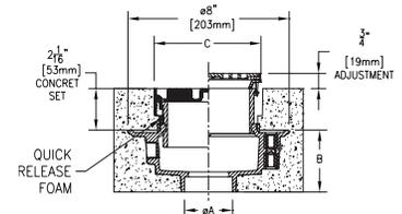
\*Cast Iron Adapter substituted for standard ABS adapter
