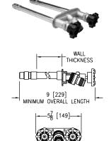
Standard inlet connection combination 1/2" [13mm] female solder x 1/2" [13mm] male IP.
