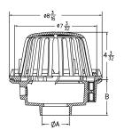
• Gravel guard manufactured from durable cast iron
