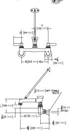
· Ceramic disc operated cast brass service sink faucet with vacuum breaker and service stops.
