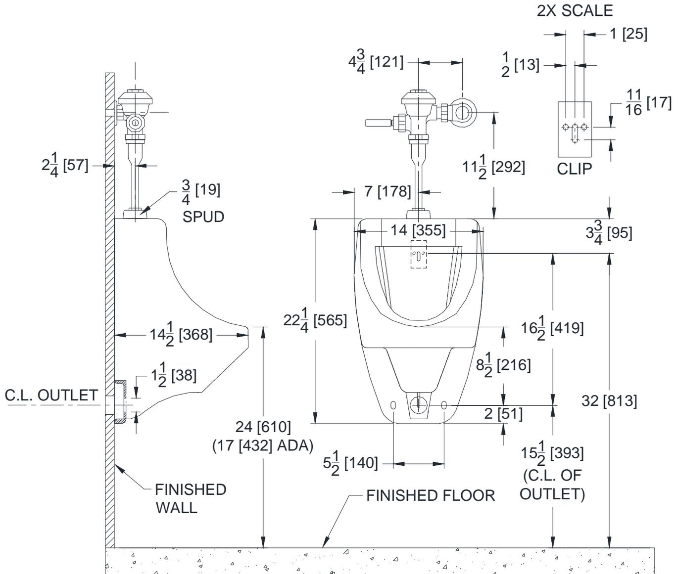
NOTE: Rough-in for concealed plate carrier, see Zurn Z1222 Rough-in sheet.
