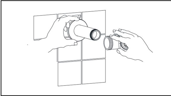
3. Insert the flush valve tailpiece into the stop valve and hand tighten the lock nut to the stop valve. Plumb the entire unit (see 3).
