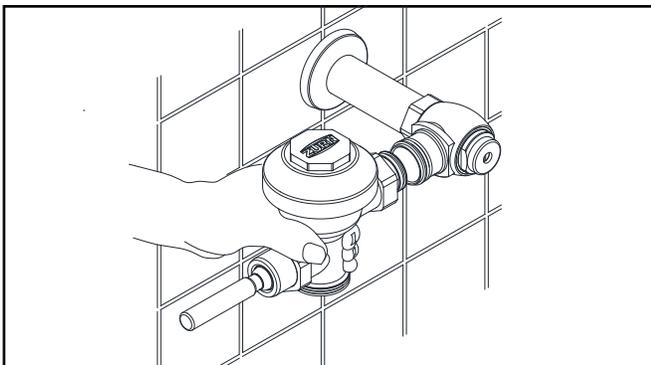
4. Determine the length of vacuum breaker tube required to join the flush valve and fixture spud. Cut the vacuum breaker tube, if re quired, to this length (see 4a). Assemble the vacuum breaker tube assembly and spud nut assembly to the flush valve and fixture spud (see 4b).
