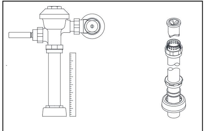
5. Hand tighten spud nut and vacuum breaker tube nut to fixture and flush valve. Adjust the valve assembly for plumb. Tighten fixture spud nut, vacuum breaker tube nut and lock nut with a wrench.
