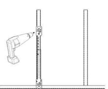
Set to desired height for box  $\mbox{\ensuremath{\mathbb{Q}}}$  . Align on stud.
