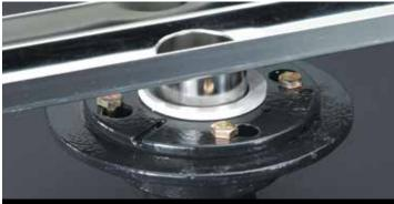
Cast Iron membrane fitting – typically used with plain body channel. Allows connection and clamping of either a fabric or CPE membrane with a compression fit. Suitable when plastic fittings are considered a fire hazard. Push-fit and threaded units available.
