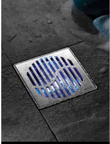
Water activated LED light unit sits below the grate and illuminates whenever the water is running. For use with deep body shower point only. Light kit includes (1) rechargeable LED pack and (1) 110v UL rated low voltage charger.
