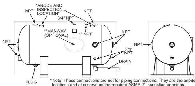
\*Note: These connections are not for piping connections. They are the anode locations and also serve as the required ASME 2" inspection openings.
