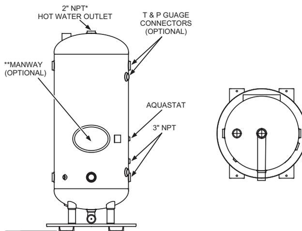
\*\*Manway standard on cement and required on tanks with bundles 48" and larger.
