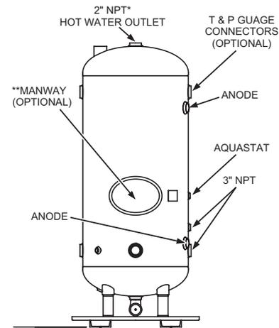
\*\*Manway standard on cement and required on tanks with bundles 48\" and larger.
