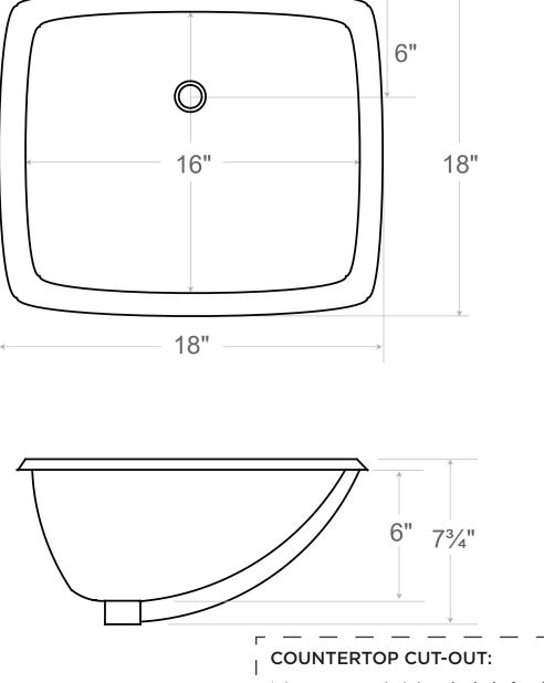
It is recommended that the hole for the sink be cut  $\frac{1}{2}$ " x  $\frac{1}{2}$ " smaller than the inside bowl dimensions.
