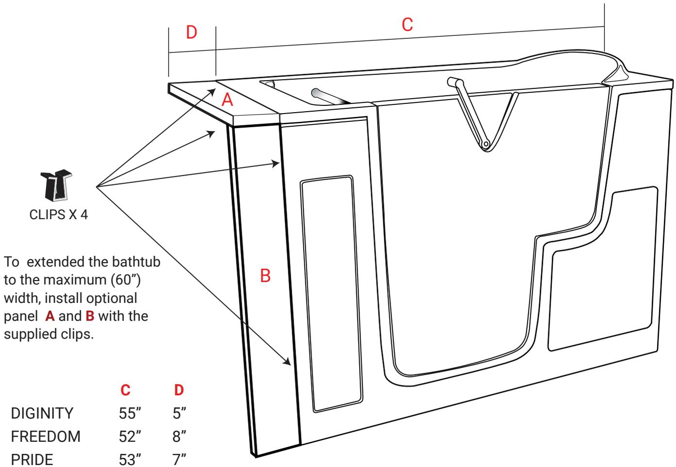
To extend the bathtub to the maximum (60") width, install optional panel **A** and **B** with the supplied clips.
