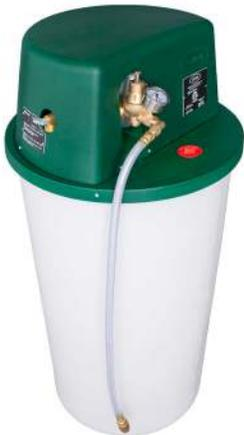
Axiom System Feeders are designed to simplify the process of maintaining the cold static fluid pressure in closed-loop heating and cooling systems. Having a reservoir of suitable make-up fluid eliminates the need for backflow prevention and helps solve many of the associated problems when using domestic water as a make-up fluid.
