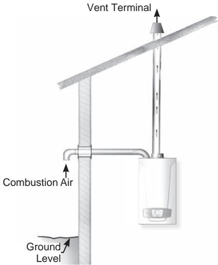
**FIGURE 6-17 - (3") Twin Pipe Roof Vent**
