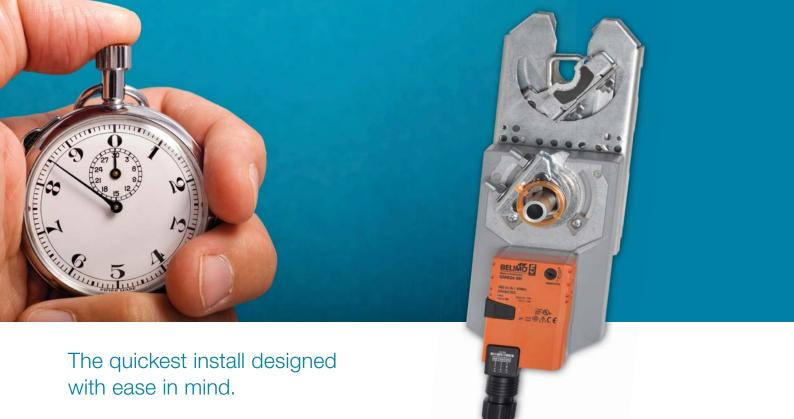
The ZG-JSL linkage is designed to facilitate the attachment of select Belimo actuators to a damper's jackshaft. The unique open ended design allows the linkage to clamp on to any part of a jackshaft measuring from 1/2" to 1.05" in diameter.
