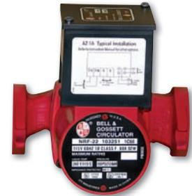
NRF-VS Pump Control is a versatile variable speed control for use in hydronic heating and cooling applications. Water temperature is controlled by regulating the speed of the pump which injects water from a different temperature water loop into a controlled loop.
