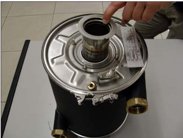
Fig. 6 Burner head
