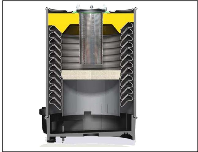
Fig. 7 Heat exchanger & Burner cross-sectional view
