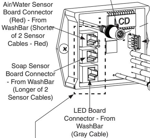
**A** Make (3) connections from the WashBar assembly as shown (Air/Water Sensor, Soap Sensor and LED)
