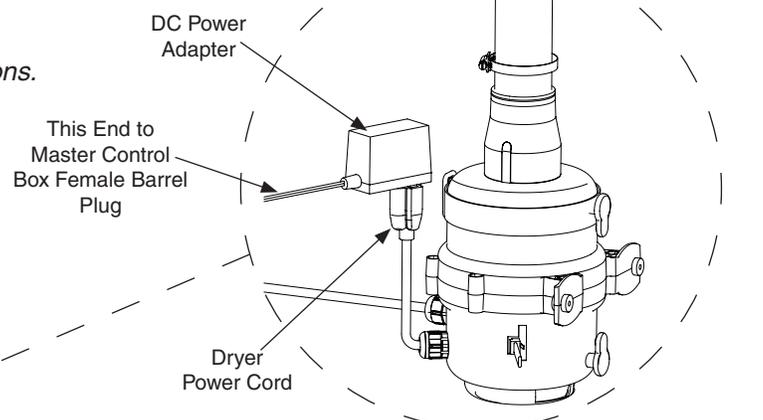
**C** Make barrel plug and connector plug connections as shown.
