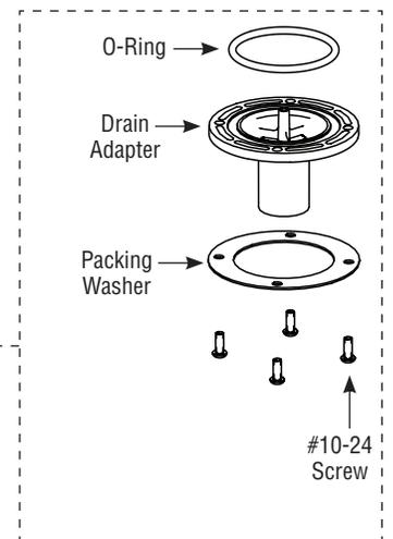
**A** Assemble the remaining components as shown and thread the four screws through the drain adapter and into the basin inserts. Ensure the screws compress the drain adapter evenly onto the basin. Do not overtighten.
