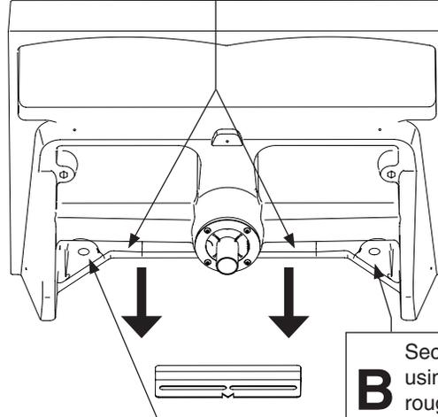
**B** Secure the bowl to the wall anchors using fasteners per the structural rough-in requirement (supplied by installer).
