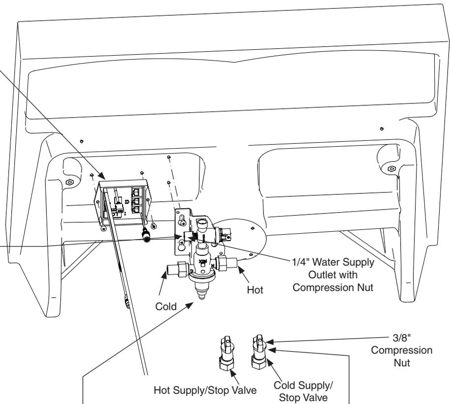
**C** For thermostatic mixing valve installation, secure 1/2" supply hose to hot water supply valve inlet. Secure the other supply hose from cold water supply to cold water supply valve inlet. Secure valve to bowl using (2) #10 x 1/2" long screws.
