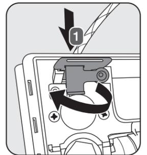
3. Be sure to seat hose firmly before reinstalling metal key and securing it with yellow locking tab.
