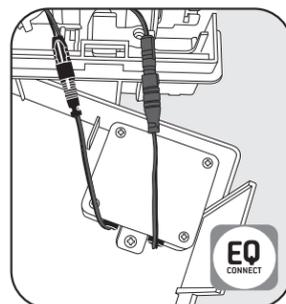
2. Attach wiring connectors located on the inside of the control box cover (gray to gray, black to black). Snap the completed connections into the wiring harness.
