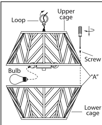
1. Tighten the loop to the stem on the fixture.
