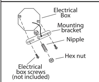
5. Loosen the upper connector from nipple. Attach the mounting bracket to the electrical box using electrical box screws (not included). Attach the nipple to the mounting bracket and adjust until it will clear the canopy when assembled (Place the canopy over the nipple and tighten the upper connector onto the nipple until snug. The upper connector should hold the canopy snug to the ceiling). Lock the nipple in the correct position using the hex nut.
