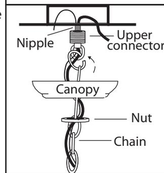
7. Loosen the nut on the upper connector and slide it down the chain towards the lower connector. Slide the canopy down the chain towards the lower connector. Feed the wire through nut, canopy, the upper connector and onto the nipple. Tighten the upper connector onto the nipple. Spread the other end of the chain open and fasten to the upper connector. Ensure the opening is closed.
