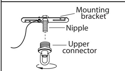
4. Determine the height that you would like to hang your fixture. Trim the cord and chain. Allow 10" of extra wiring for the electrical box connections.
