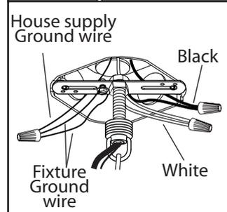
8. Connect the ground wires (bare copper or green) from your fixture to the ground wire (bare copper or green) or ground screw in the electrical box. Connect the black wire (or wire marked "SPT-1") from the fixture to the black wire in the electrical box and connect the white wire (or the wire with ribbed side) from the fixture to the white wire in the electrical box.
