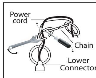
6. To attach chain loop to light fixture, use a screwdriver and wrench to open and close chain loop. Ensure to close the opening. Weave the power cord and ground wire through the links in the chain.
