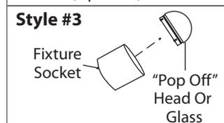
**Style #3** - Snap "pop off" head or glass onto fixture (push, or push and turn (it depends on the style of your fixture)). Install proper bulb type and wattage (not included).
