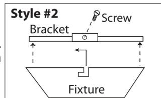
**Style #2** - Insert one screw into the mounting bracket - do not tighten yet. Tuck electrical wires into outlet box and position fixture over the mounting bracket. Line up the screw in the bracket to to the "7" hole on the fixture. Slide fixture to secure in place. Insert remaining screw. Tighten both screws to secure.
