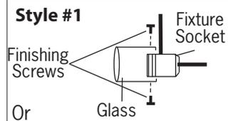
**5. Style #1** - Install proper bulb type and wattage. Remove the finishing screws that are already on your fixture. Position glass in place and secure with finishing screws. Install the proper bulb type and wattage (not included).
