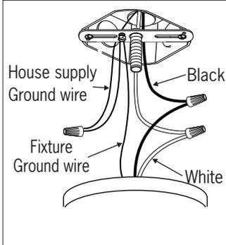
**4.** Once connections of wires are completed, carefully tuck wires and wire nuts into the outlet box making sure no bare wire (on the black and white) is visible at the wire nuts.
