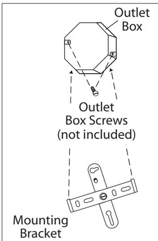
**1.** Mount the mounting bracket to outlet box using outlet box screws (not included). Make sure the studs or nipple on the mounting bracket are facing out from the outlet box.
