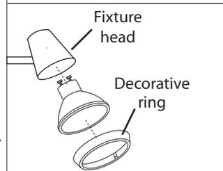
**6.** Install proper bulb type and wattage (not included). Install decorative ring.
