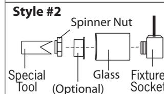
**Style #2** - Remove spinner nut from the socket. Place the glass onto the fixture socket. Use the special tool that comes with your fixture to tighten the spinner nut onto the socket to secure the glass in place. Install the proper bulb type and wattage (not included).
