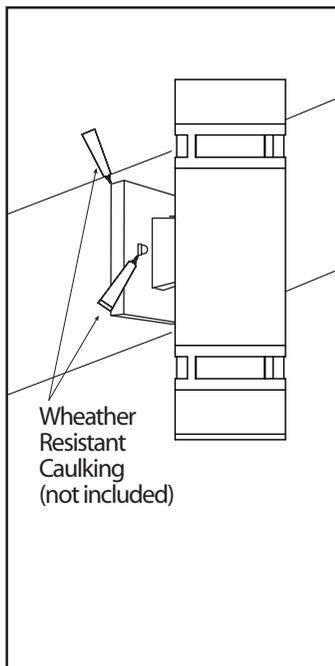
After Installation, seal around the top and side perimeter between the fixture and the wall surface with weather resistant caulking. The bottom should be left un-caulked to prevent moisture build-up. Apply a small amount of weather resistant caulking around the side perimeter between the cap nut and mounting plate.
