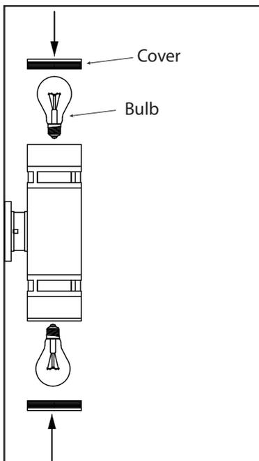
Install specified bulb type and wattage (not included). Push covers onto the fixture.
