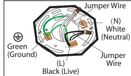
For multiple black (live) & white (neutral) wires joined in the electrical box (house wiring), attach a single "black" and "white" Jumper Wire before connecting. Strip 7mm from a 6" Jumper Wires (AWG 12-24) supplied. Then connect (push) wires into correct inserts.
