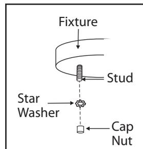
Once wire connections are completed, carefully tuck wires and wire nuts into the electrical box making sure no bare wire (on the black and white) is visible at the wire nuts. Position fixture over studs on mounting bracket assembly. Secure fixture in place with star washers and cap nuts.
