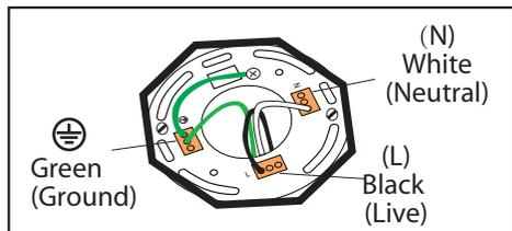
Connect (push) electrical wires from electric box (house wiring) into correct inserts. Black (Live), White (Neutral), Green (Ground)
