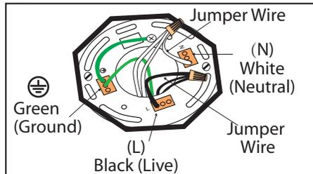
For multiple black (live) & white (neutral) wires joined in the electrical box (house wiring), attach a single "black" and "white" Jumper Wire before connecting. Strip 7mm from a 6" Jumper Wires (AWG 12-24) supplied. Then connect (push) wires into correct inserts.
