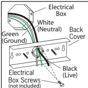
Attach easy connect mounting bracket to electrical box with electrical box screws (not included).
