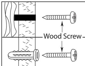
Additional support may be required for fixtures longer than 20". Position the fixture and add wood screws (one on each side) for the wooden studs or plastic wall anchor and wood screws for dry wall.
