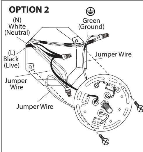
Option 2: For multiple green (ground), black (live) and white (neutral) wires joined in the electrical box (house wiring), attach a single "green", "black" and "white" jumper wire before connecting. Dress Black, White, Green wires through supplied holes in bracket. Strip 7mm from a 6 in. jumper wires (AWG 12-24) supplied. Then connect (push) wires into the correct inserts.
