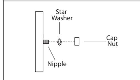
**4.** Once connections of wires are completed, carefully tuck wires and wire nuts into the electrical box making sure no bare wire (on the black and white) is visible at the wire nuts. Position hole in fixture over nipple and secure in place with star washer and cap nut.
