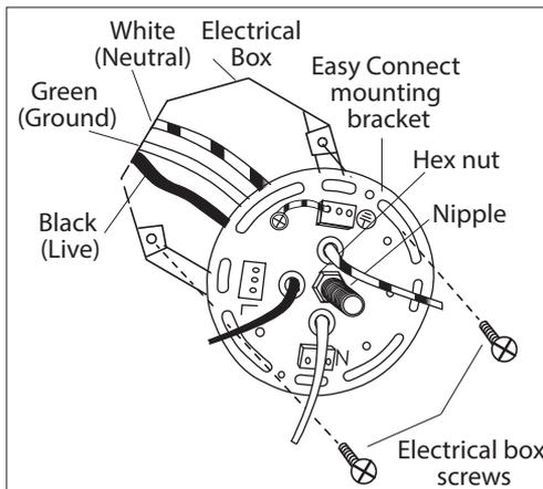
**1.** Attach nipple to mounting bracket. Adjust so it will clear hole in back of fixture and then lock nipple in place with hex nut. Dress Black, White, Green wires through supplied holes in bracket. Attach mounting bracket to electrical box with electrical box screws (not included).
