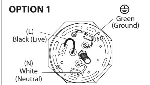
**2.** Option 1: Connect (push) electrical wires from electric box (house wiring) into correct inserts.
