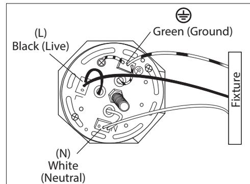
**3.** Connect (push) electrical wires from fixture into correct inserts.
