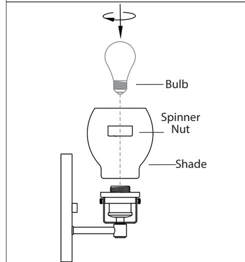
**5.** Remove spinner nut from socket. Position shade on lamp and secure with spinner nut.
