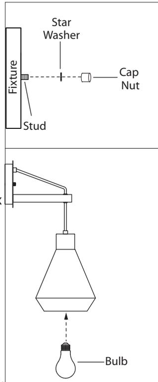
**4.** Tuck electrical wires into electrical box and position fixture over studs on mounting bracket assembly. Secure fixture in place with star washers and cap nuts.
