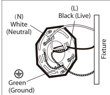
**3.** Connect (push) electrical wires from fixture into correct inserts.
