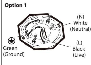
**2. Option 1:** Connect (push) electrical wires from electric box (house wiring) into correct inserts.
