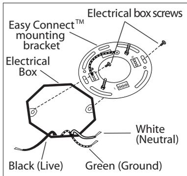
**1.** Attach Easy Connect™ mounting bracket to electrical box with electrical box screws (not included).
