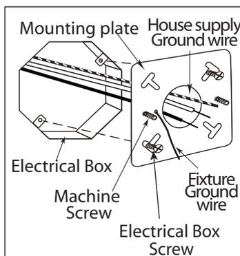
4. Remove knockouts (on the mounting plate) corresponded to the mounting screws on the electrical box.
