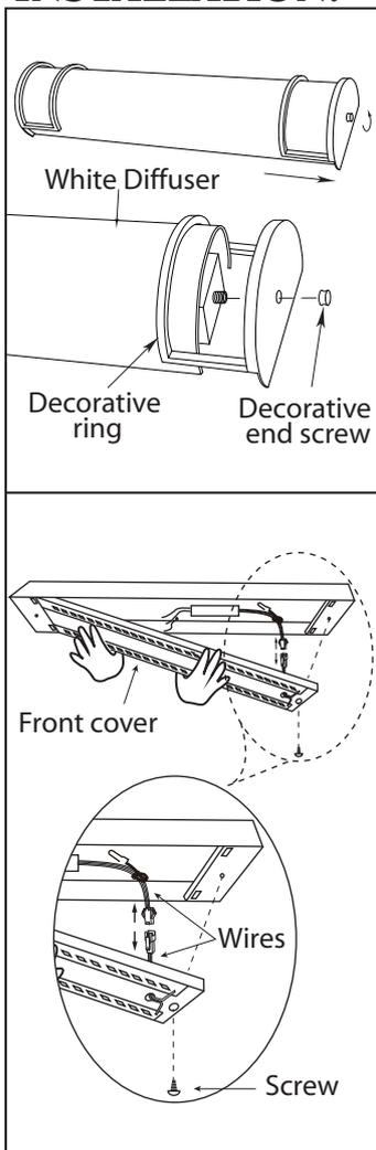
1. Remove the screw on the both sides.
