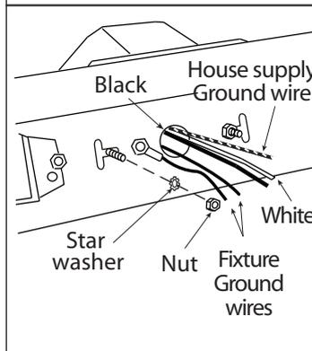
5. Tighten the back plate over the mounting plate by the star washers and nuts provided. Ensure the back plate is level to the floor. Additional support may be required for fixtures longer than 30". Position the fixture and add wood screws (one on each side) for the wooden studs or plastic wall anchor and wood screws for dry wall.
