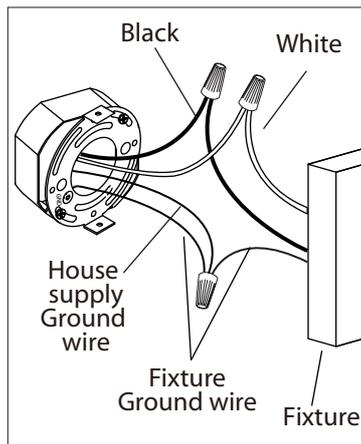
**3.** Connect the ground wires (bare copper or green) from your fixture to the ground wire (bare copper or green) or ground screw in the electrical box. Attach the black wire from the light fixture to the black wire in the electrical box. Attach the white wire from the light fixture to the white wire in the electrical box.
