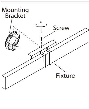
**1.** Remove the mounting bracket from the fixture by unscrewing the 2 screws.
