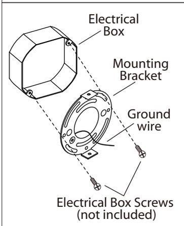
**2.** Mount the mounting bracket to electrical box using electrical box screws (not included).
