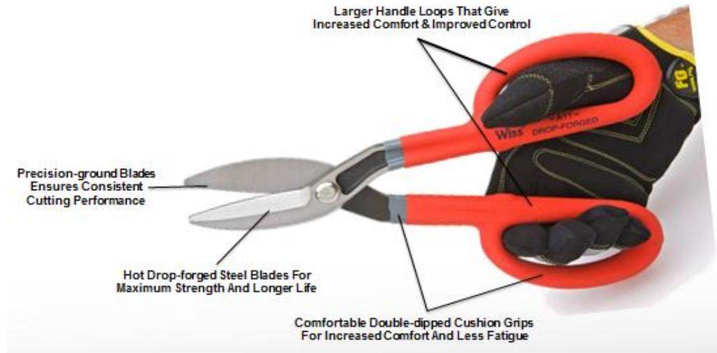
Duckbill Blades Design On V10N & V19N Snips Facilitates Tight Circular Cuts
