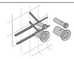
**STEP 8:** Install two 1/2" x 6" fixture support rods with plastic sleeves (C), the pipe caps (D) and mud guard (E) are mounted for protection during wall surface construction, see fig. [7].
