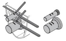
**STEP 9:** FiberBond wallboard, 1/2" tile backer board or plywood with a ceramic tile surface would be most suitable materials recommended for wall finish in order to support the wall hung toilet bowl. Holes in wallboard for ceramic bolts must be 1" (25).
