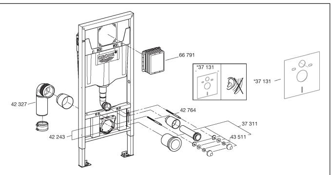
The tank and carrier are designed to fit within a 2" x 6" wood frame (or equal) construction. The studs must be placed 19-11/16" apart at the location where the unit will be positioned prior to installation into the wall. The carrier legs must be adjusted for the finished rim height of the water closet bowl. The dimensions may be taken from the bowl or from the specification sheet. Be sure to allow for finished floor covering.
