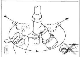
**5.** Use a correctly sized open-ended spanner to tighten. Do not use stillsons, etc, or over-tighten
