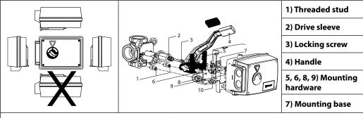
When installing the handle (4), it should be installed opposite to the indicator on the drive sleeve and the end of the handle should be facing away from the valve. Failure to properly install the handle will result in damage to the 90 series motor actuator due to the interference of the mounting stud (1) with the rotation of the handle
