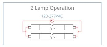
**NOTE**: both pins on each end of lamp must be connected to line voltage as shown above. If lamp holder is a "non-shunted" (T12) type, it must be shunted (shorted) by external jumper. Most T8 lamp holders are internally shunted and will not require an external jumper.
