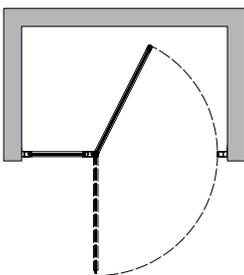
**NOTE:** Inward opening and entry can be compromised by insufficient depth of enclosure. Call customer service for more information.
